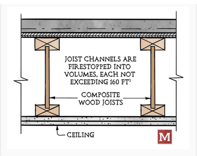
As stated, the requirements of 8.15.1.2.6 are only specific to whether sprinklers can be omitted from a combustible concealed space. Section 11.2.3.1.5 must also be considered. This section requires the adjacent area of sprinkler operation to be 3,000 square feet unless one of the exceptions found in 11.2.3.1.5.2 are met.
